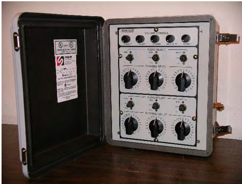
DICES Sub-MUX Hazardous Area Operator Station
