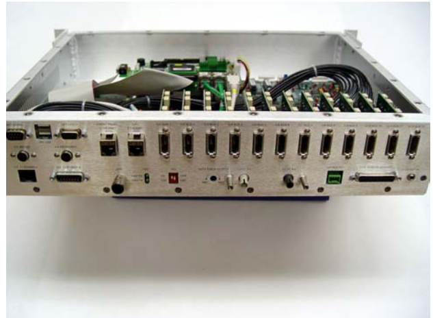
Rear panel of STRATCOM station showing the twelve secure audio inputs across the upper panel, each with isolated input card mounted inside and mated to other station electronics.
